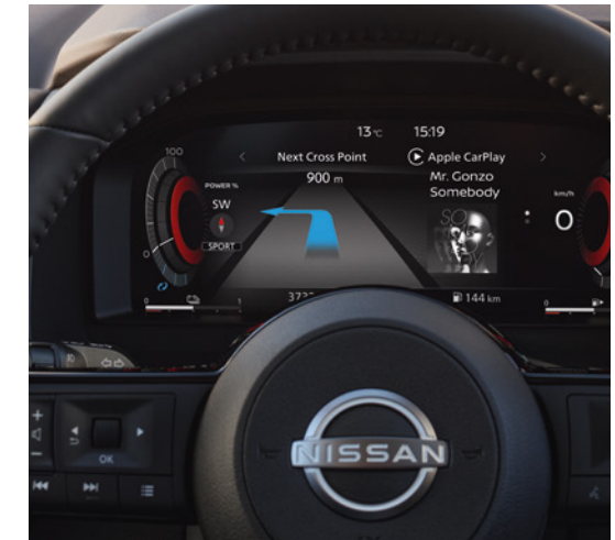
12.3" Fully digital meter* 10.8" Windscreen Head-up display*
